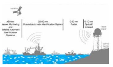
Figure 04: A snapshot of an Integrated Surveillance System
